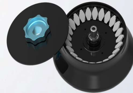
CR-15-24 Fixed angle rotor of 1544R for 24 1.5mL/ 2.0mL microtubes
